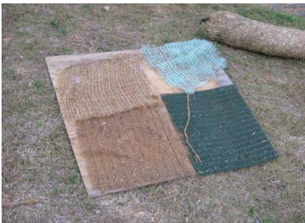
*A display of commonly used erosion control products.*
