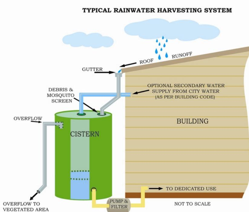
**Cistern** – The cistern is the above ground or buried tank that holds the rainwater until it is used. It can be made from various materials; typically plastic or metal.
