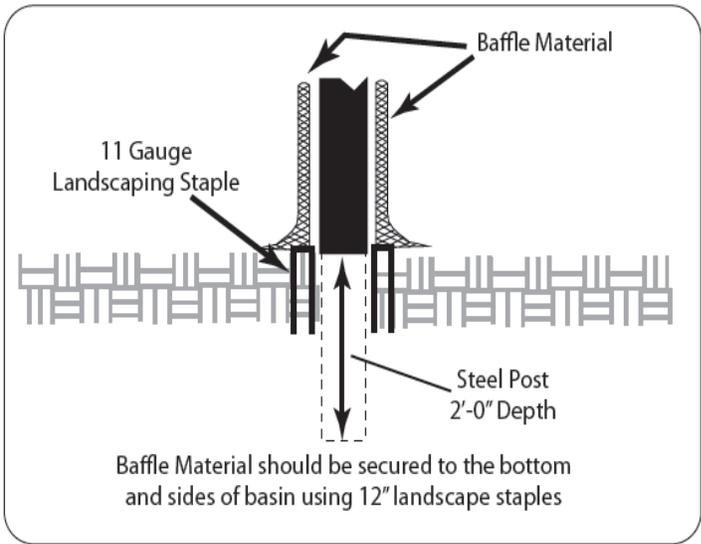
**Figure 6.65b Coir Fiber Baffle Detail**
