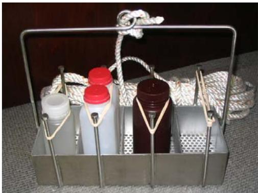
**Figure 2. Cage sampler used in the DWQ Ambient Monitoring System**
