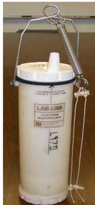
**Figure 4. Labline sampler for photic zone measurements.**
