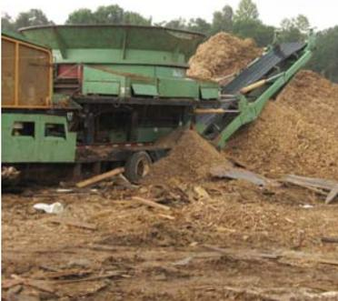
**A tub grinder is used to process clean wood waste into boiler fuel.**
