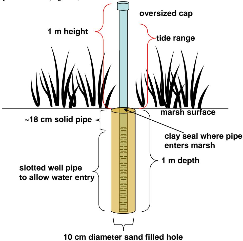
Figure 5: Groundwater well design. Instruments placed inside well pipe measure temperature, salinity, and water level.
