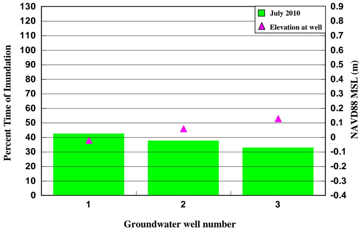
Figure 14: Middle Marsh inundation plot based on water level meters. Pink diamonds indicate marsh surface elevations at each groundwater well. Well 1 is nearest the water, well 3 is the farthest from the water.
