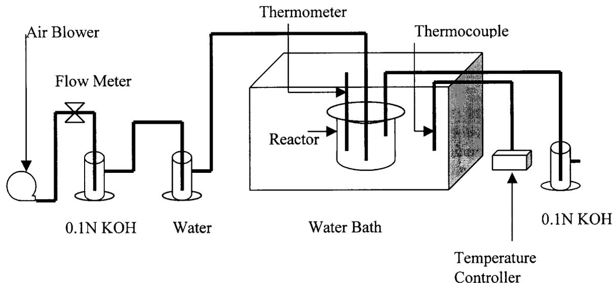
**Figure 1.** The laboratory scale reactor.
