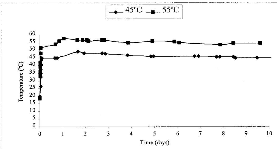
**Figure 2** Temperature changes in MSW mixed with MDF sawdust composting reactor under fixed temperature controls
