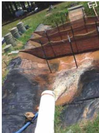
Figure 1. Photo of stilling basin beginning to fill.
