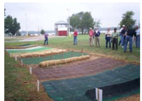
*Turf reinforcement matting displayed here along with different types of diversions, including triangular silt dikes, straw wattles, and coir wattles.*
