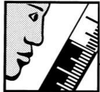
*Let the stick gently touch bottom, and quickly bring it back up. Read the depth of the fuel indicated by the wet mark on the stick to the nearest 1/8 inch.*
