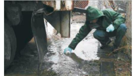
Stormwater sample being collected. Sample should be taken at SDO, which is typically at the lowest point before water leaves the property.
