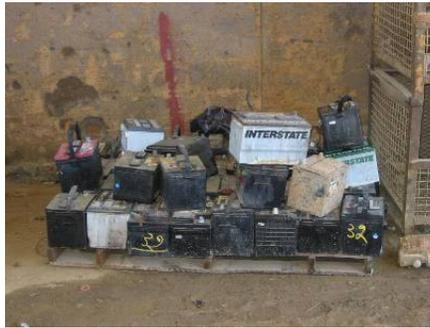
Example BMP showing batteries stored above ground (on pallet) and under cover (inside storage building)
