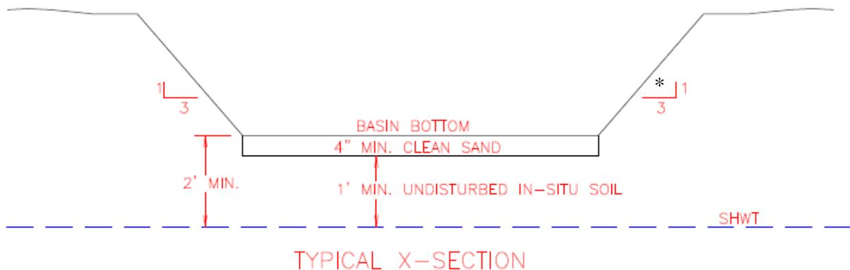
\*Retaining walls may be used in place of the 3:1 vegetated side slopes.
